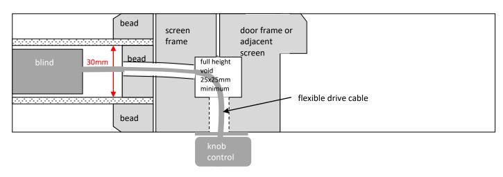
30mm cavity between glass is the only critical dimension, all others as you would normally for timber screen
